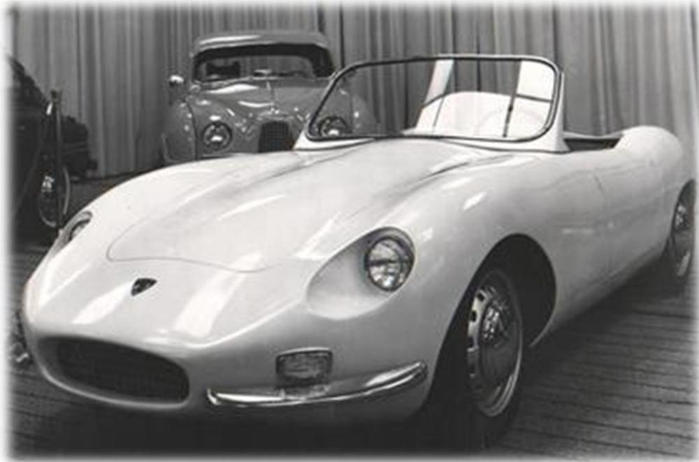
*Offset front view of the Saab Quantum with its very stylish glass-fibre body-shell.*
